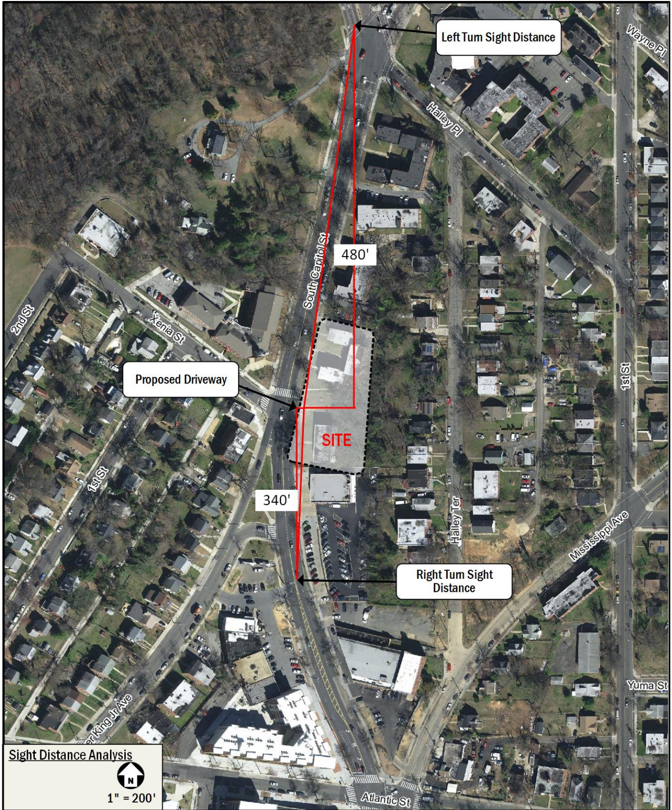
Figure 11: Sight Distance Analysis
